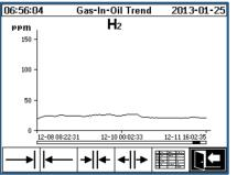
A graph displaying the trend over the time, in this case Hydrogen (H<sub>2</sub>), is shown.
